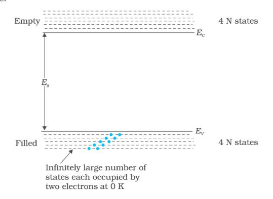
The energy band positions in a semiconductor at 0 K. The upper band, called the conduction band, consists of infinitely large number of closely spaced energy states. The lower band, called the valence band, consists of closely spaced completely filled energy states.
